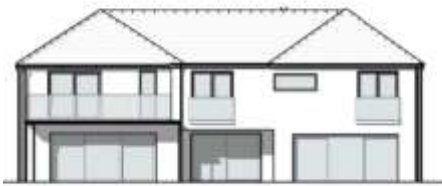
03 PROPOSED REAR ELEVATION 1:100
