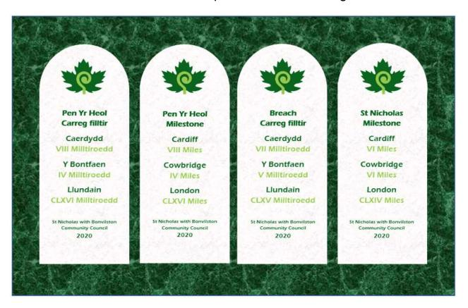
Four casts would be required, costing £400 each. The lettering and numbering imprinted into the concrete, and filled with a green resin. These would them be situated where the original milestones were placed.
